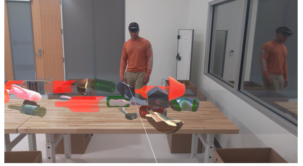
Figure 4: The dangerous objects—such as broken glass bottles or metal cans—are highlighted among the debris of the rest of the recycling material.
