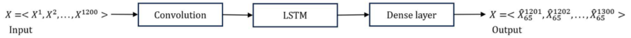
Fig. 2. CNN-LSTM hybrid architecture (10s model), displaying the output of a single confidence value sequence (65 th feature).
