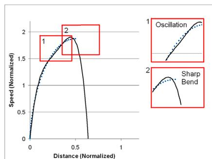
Figure 3. Fitting issues with a quartic polynomial include undesirable oscillation (1) and sharp bends rather than smooth continuity (2).
