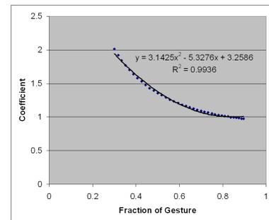
Figure 10. Quadratic curve fit to coefficients that are used to correct our endpoint location.
