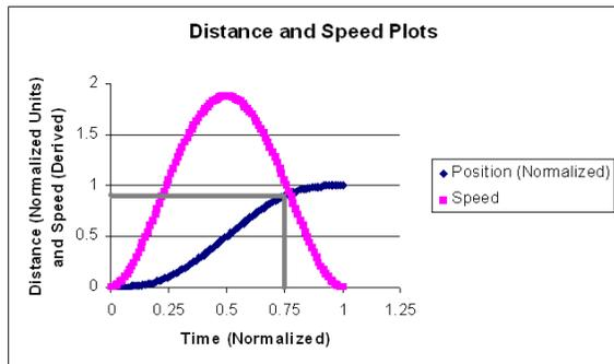
**Figure 1. Theoretical distance and speed versus time profiles predicted by the Minimum Jerk Law.**
