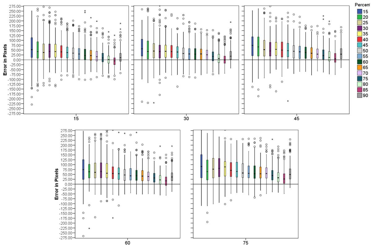
Figure 5. Predictive accuracy of our algorithm at locations along gesture path. Gesture path percentage is estimated based on  $\frac{\text{distance\_traveled}}{\text{predicted\_endpoint}}$ .
