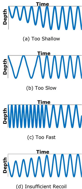
**Figure 3.** Compression motion, i.e., the up-and-down motion that the avatar's hands make while performing compression gestures.
