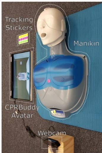
**Figure 2.** CPRBuddy's components.
